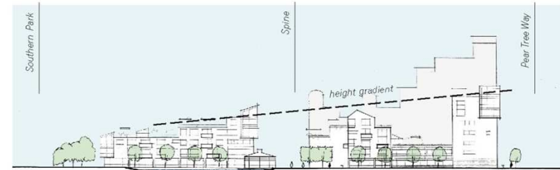
Figure 35: Section AA through community square, indicating volumetric variation and east/west height gradient over Phase 3.
